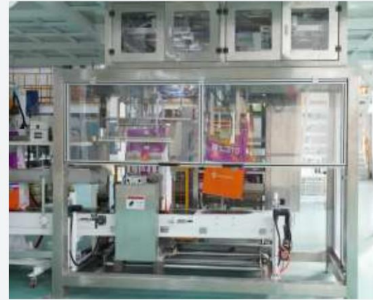
Ensures correct package shape before palletizing.
