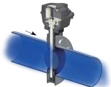
Valve open status
