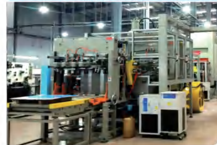
Two-pieces Can production Line
